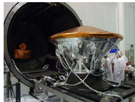
ESA’s ExoMars 2016 mission’s Schiaparelli lander undergoing thermal tests in June.
